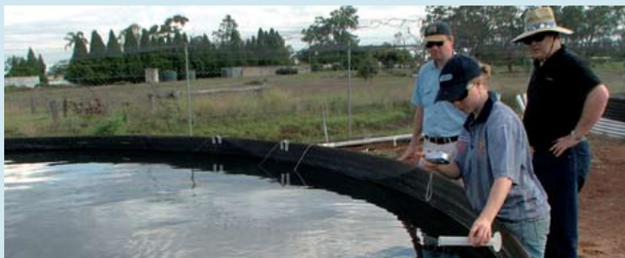
Researchers apply a monolayer to a trial site to observe evaporation reduction, photo courtesy of the CRC for Irrigation Futures
