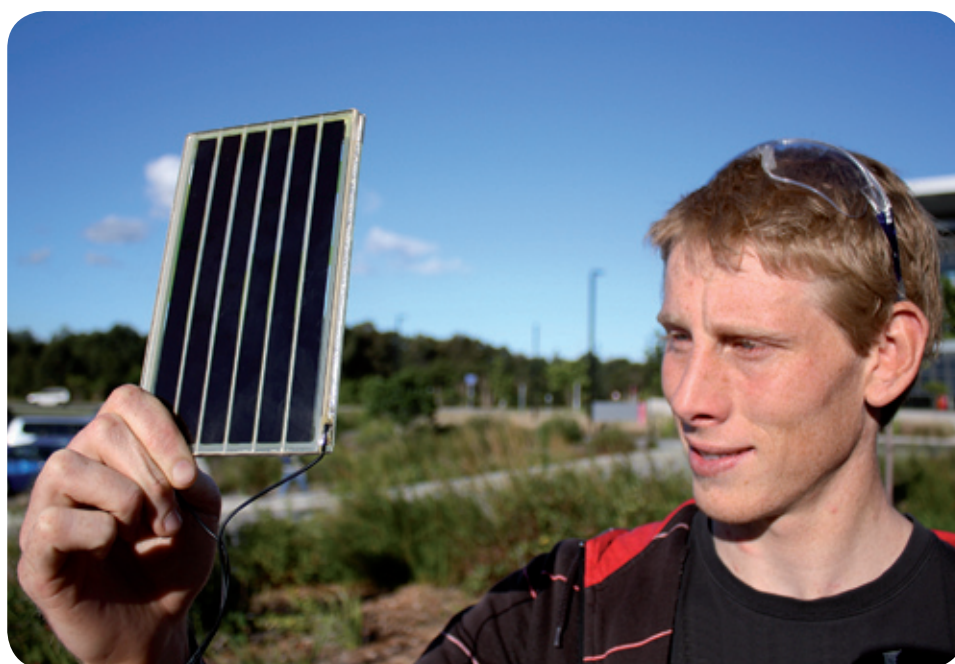
CRC for Polymers PhD student Jared Barnes demonstrates a non-silicon photovoltaic device.
